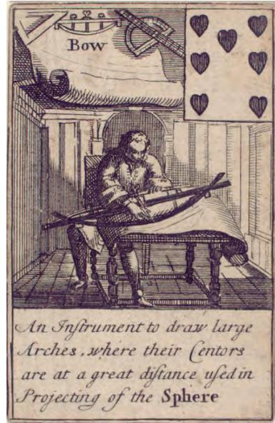
An Instrument to draw large Arches, where their Centers are at a great distance used in Projecting of the Sphere
